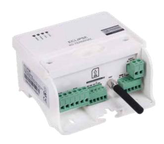
Configuring and reconfiguring, parameter changes etc. can be done via serial interfaces locally or over 3G/4G remotely. During the communication, it will initiate ID and password control/authentication.
